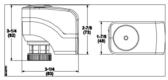
Figure 7. Dimensions of the SSA/P Series Actuator in Inches (mm).
